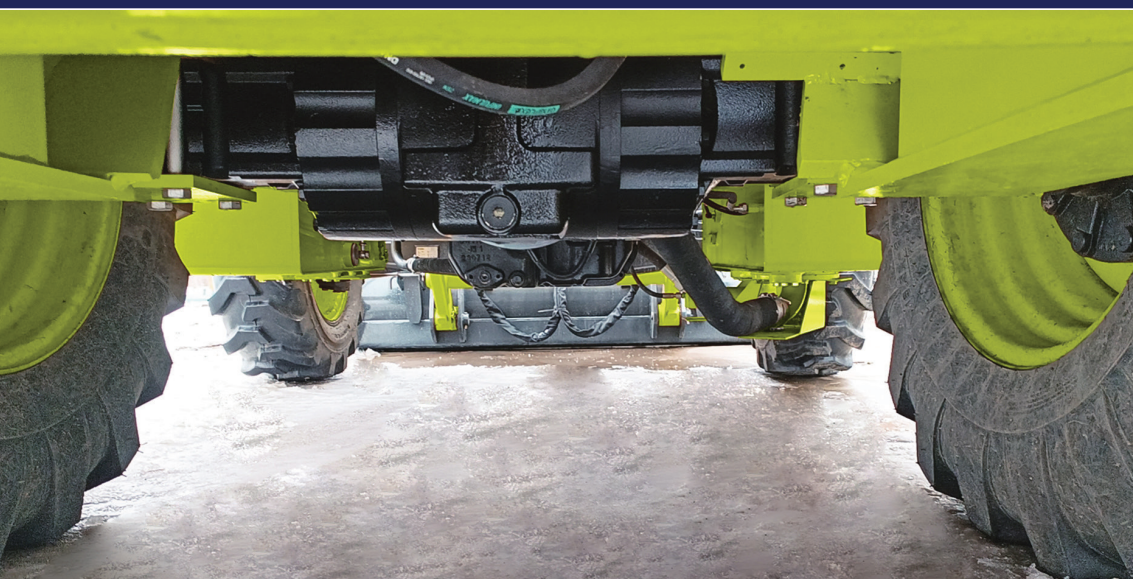
Powerful and reliable powertrain - Wet axle Core transmission technology can handle a variety of complex environments
